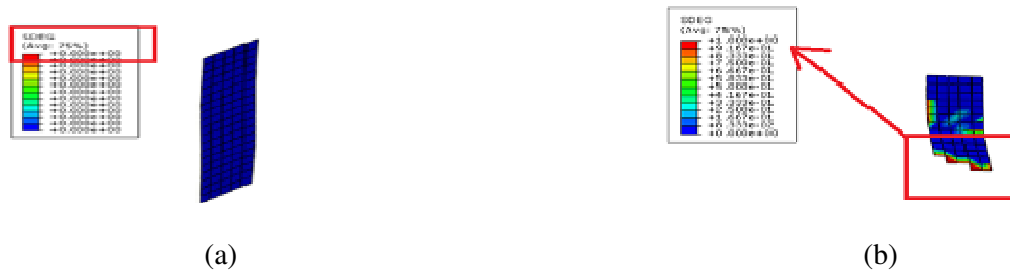
Fig.13. (a)No adhesive layer damage on S1 strengthening beams -(b)Adhesive layer deletion of S2 strengthening beams
