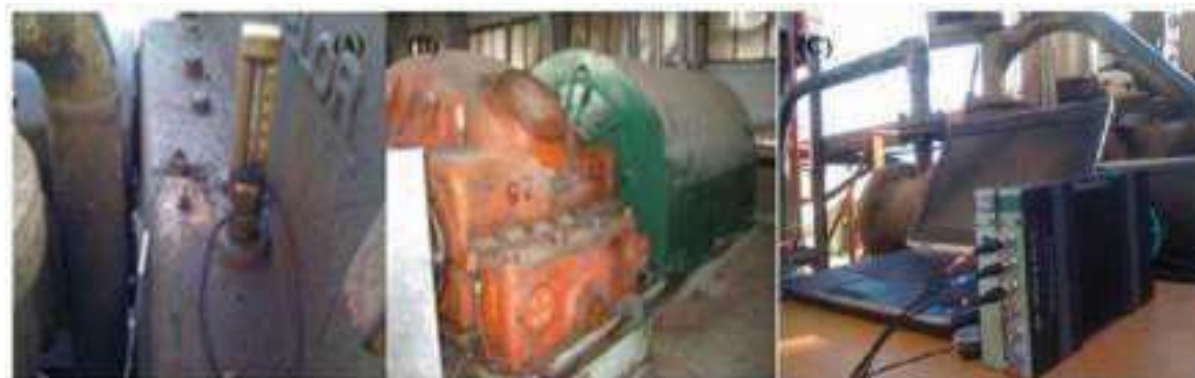
Fig. 2. Monoaxial and triaxial accelerometer (A), turboalternator (B), Pulse analyzer type 3160-A-042 (C).
